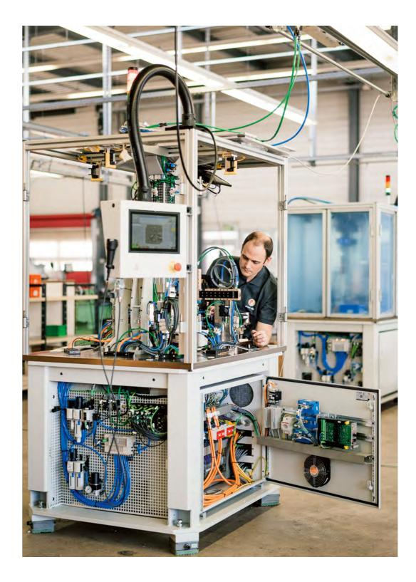
Any customer's specification will be realized, for instance, by utilizing the in-house design and construction of automatic assembly machines for contacts and connectors.
