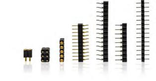
A full range of board-to-board connectors, from one to three rows of contacts, with various board terminations (SMT, tail, press-fit) using various pitch configurations (1 mm, 1,27 mm, 2 mm, 2,54 mm). These connectors are integrated within many industrial applications for power and signal connections.
