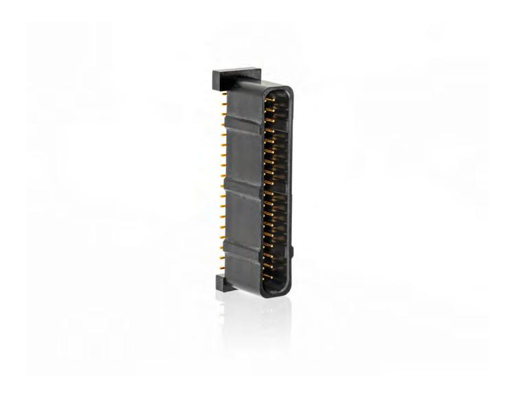
36-way, surface mount "gull wing" connectors for Electric Vehicles (EVs), assembled in our fully automated production system, ensuring stringent, highly controlled 0.10 mm coplanarity throughout the length of the connector. This connector is integrated within the inverter of the EV's power system.
