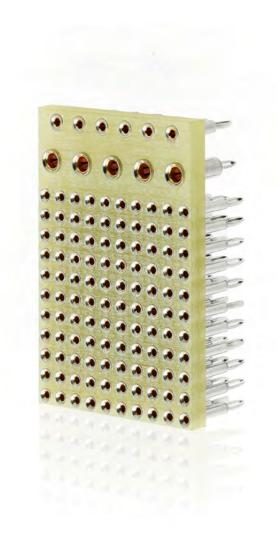
Press-fit multi-pin socket connectors, with mixed signal and power layout. These solderless connectors are integrated within the avionic electronic modules. High reliability and durability are ensured via the multi-contact point clip socket, and reliable elastic press-fit tails.
