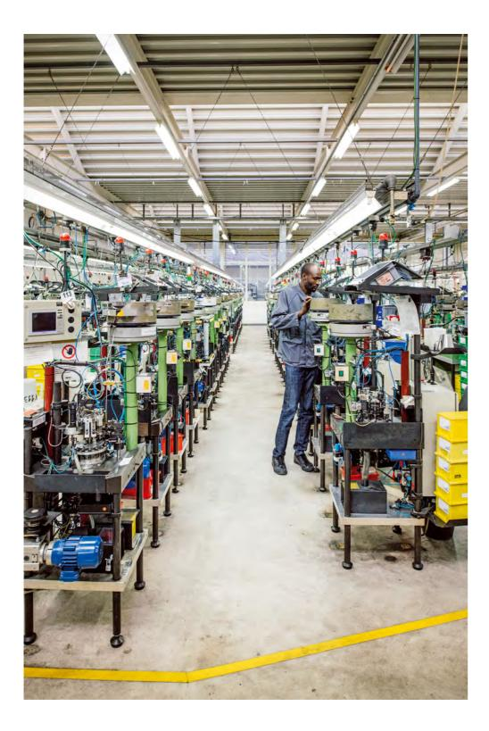
80 automatic contact assembly machines press-fitting clips within contact housings at a rate of 120 pcs./min.
